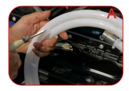
**A.** Use tools to loosen the cable tie on the fire tube and plan a suitable installation location according to the length of the tube.
