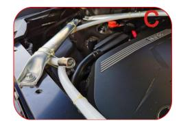
**C.** Tie the fire tube to the engine compartment with cable ties, and cut off the excess tail of cable ties.
