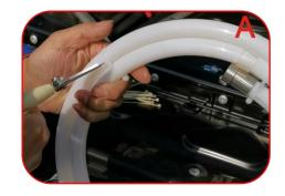
**A.** Use tools to loosen the cable tie on the fire tube and plan a suitable installation location according to the length of the tube.
